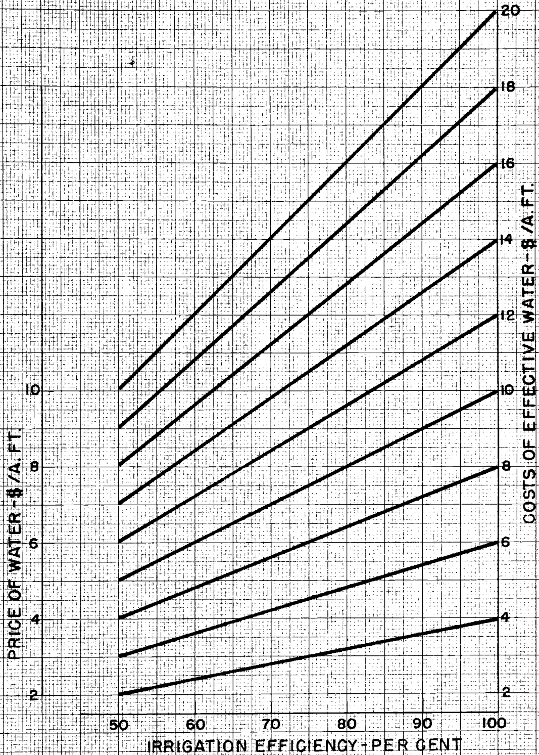
Figure 4. Costs of effective water (i. e., the water which is available for consumptive use by plants) for different water prices and irrigation efficiencies.
